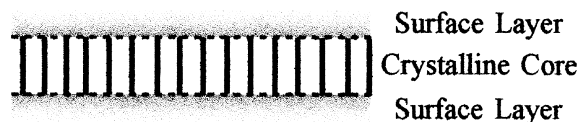
Fig. 6. Schematic drawing for the edge-on view of the POM folded-chain lamellae. The central region represents the crystalline core and the vertical thick bars illustrate the chain stems. The shaded region represents the surface layer, which contains the fold parts of chains.
